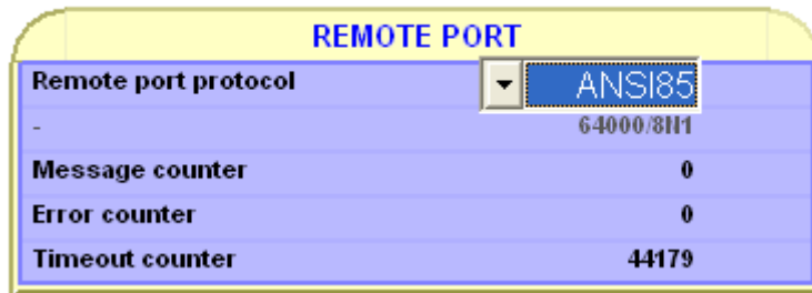
Figure 5.18: Enabling line differential communication
