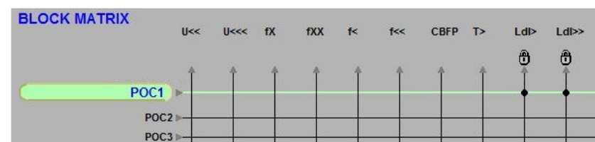
Figure 6.70: Using the block signal for differential protection blocking
