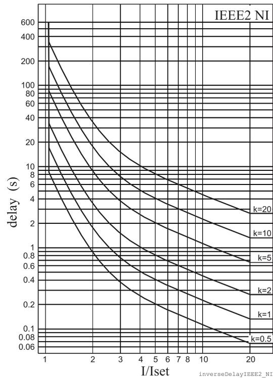
Figure 5.54: IEEE2 normal inverse delay
