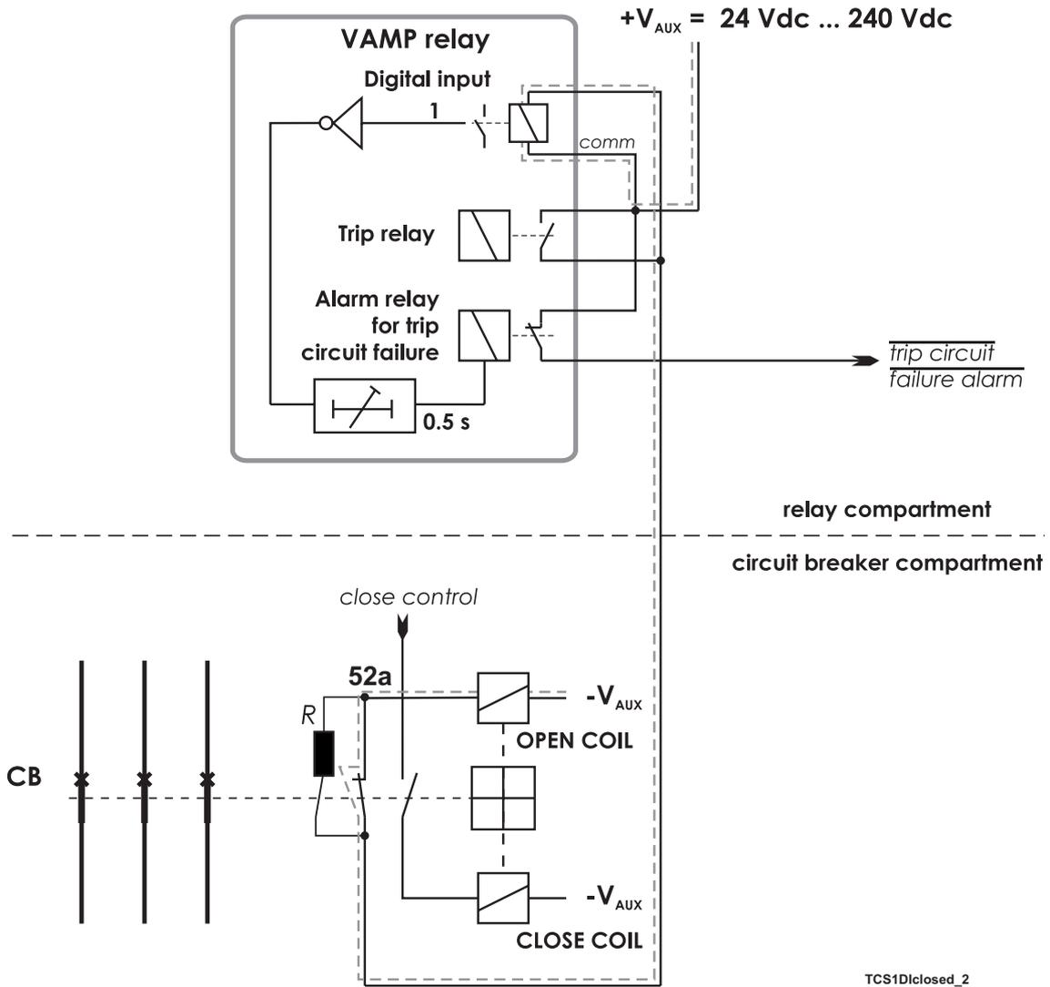
Figure 10.3: Alternative connection without using circuit breaker 52b auxiliary contacts. Trip circuit supervision using a single digital input and an external resistor R. The circuit-breaker is in the closed position. The supervised circuitry in this CB position is double-lined. The digital input is in active state when the trip circuit is complete.
