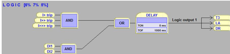
Figure 8.8: Logic can be found and modified in “logic” menu in VAMPSET setting tool
