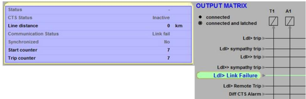
Figure 5.27: Communication failure
