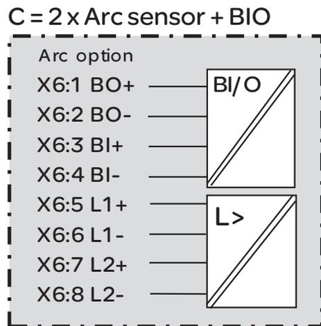
Figure 11.6: Block diagram of optional arc protection card C = Arc (2 x Arc sensor + BIO)
