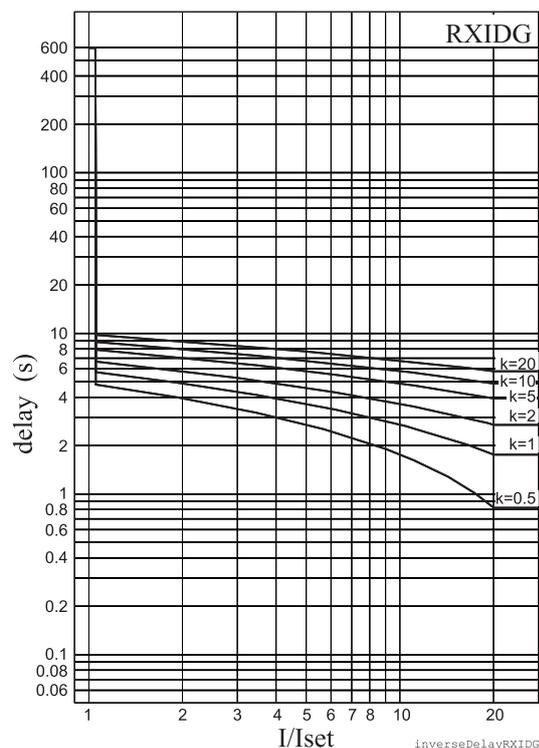
Figure 5.58: Inverse delay of type RXIDG.
