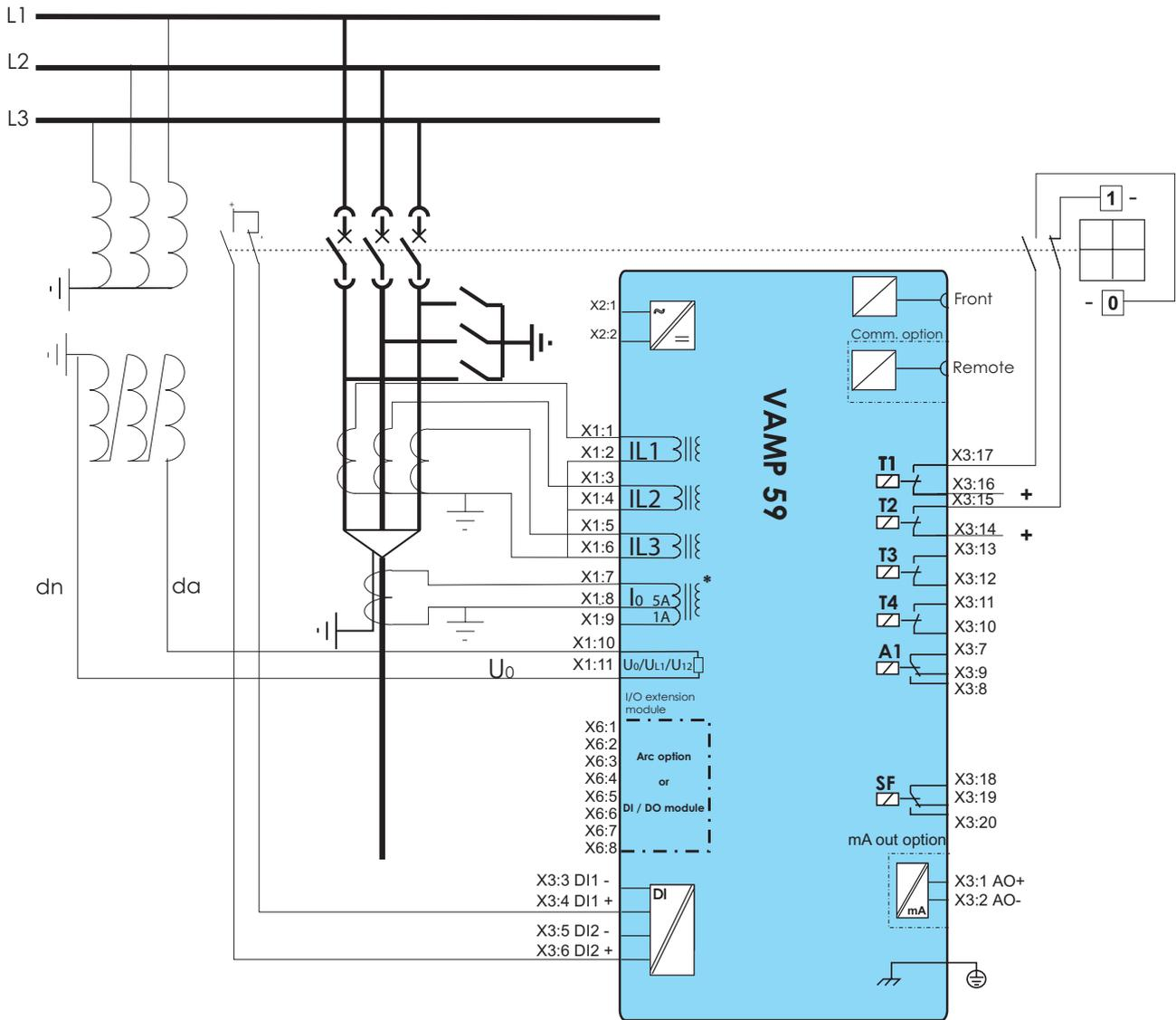
Figure 11.8: Block diagram of overcurrent and earthfault protection relay VAMP 59.
