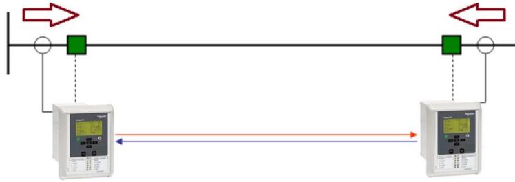
Figure 5.25: CT wiring towards the line
