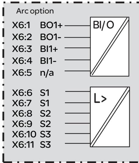
Figure 11.7: Block diagram of advanced optional arc protection card D = Advanced Arc (3 x Arc sensor + BIO)
