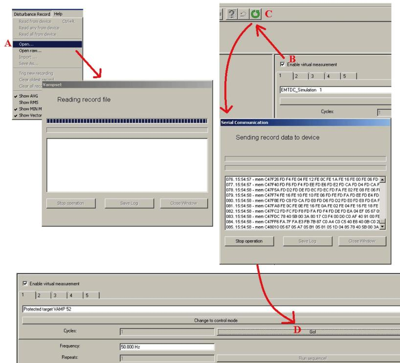
**NOTE:** The sample rate of the comtrade file has to be 32/cycle (625 micro seconds when 50 Hz is used). The channel names have to correspond to the channel names in VAMP relays:  $I_{L1}$ ,  $I_{L2}$ ,  $I_{L3}$ ,  $I_0$ ,  $U_{12}$ ,  $U_{23}$ ,  $U_{L1}$ ,  $U_{L2}$ ,  $U_{L3}$  and  $U_0$ .
