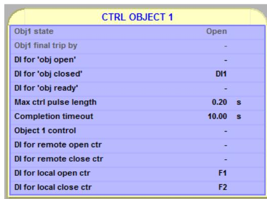
Selected object and control is shown in VAMPSET software under the menu "FUNCTION BUTTONS". If no object with local control is selected '-' is shown. If multiple local controls are selected for one key '?' is shown.
