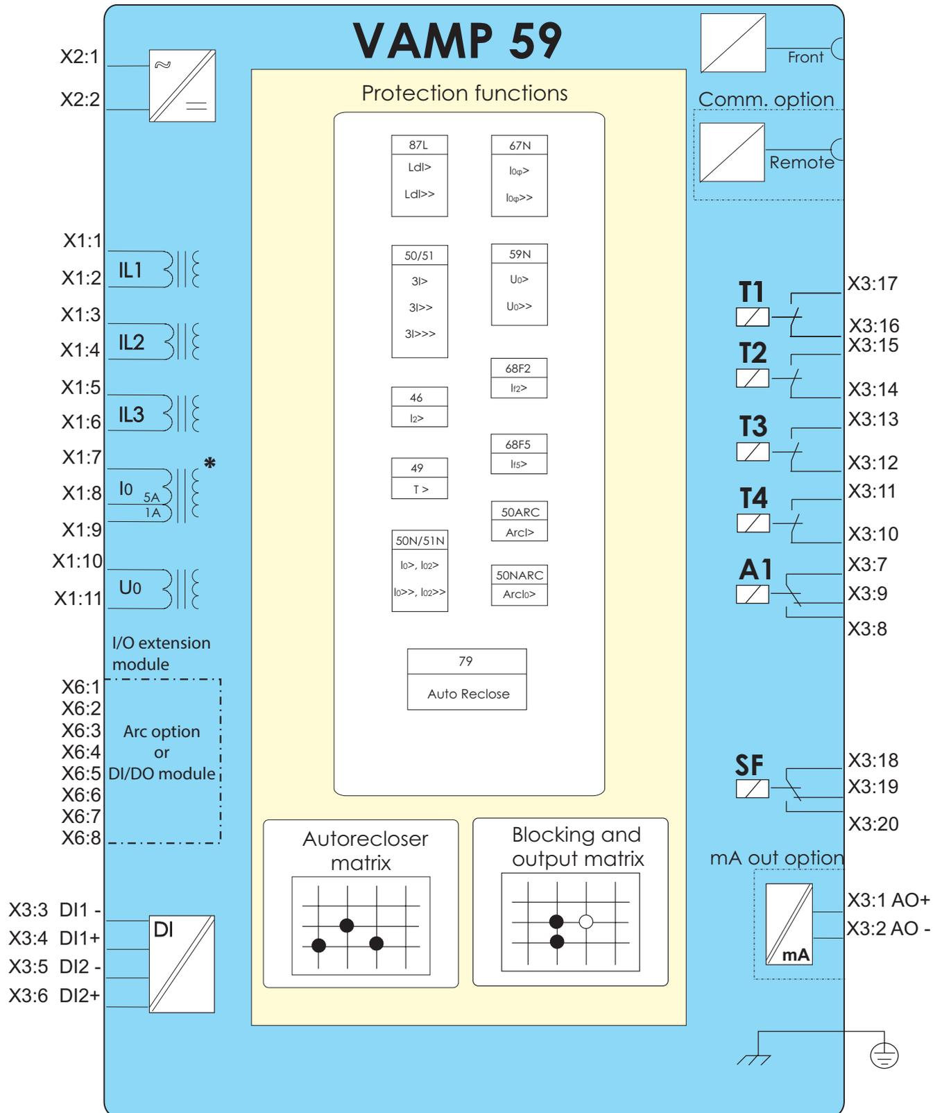
Figure 11.4: Block diagram of overcurrent and earthfault protection relay VAMP 59.
