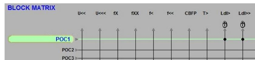
Figure 5.33: Using the block signal for differential protection blocking
