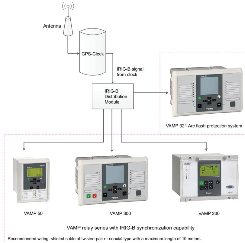
The recommended cable must be shielded and either of coaxial or twisted pair type. Its length should not exceed a maximum of 10 meters.
