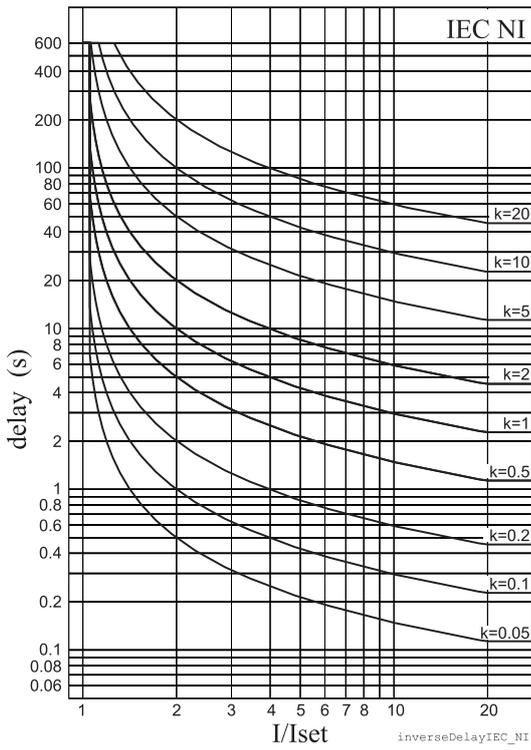
Figure 5.43: IEC normal inverse delay.
