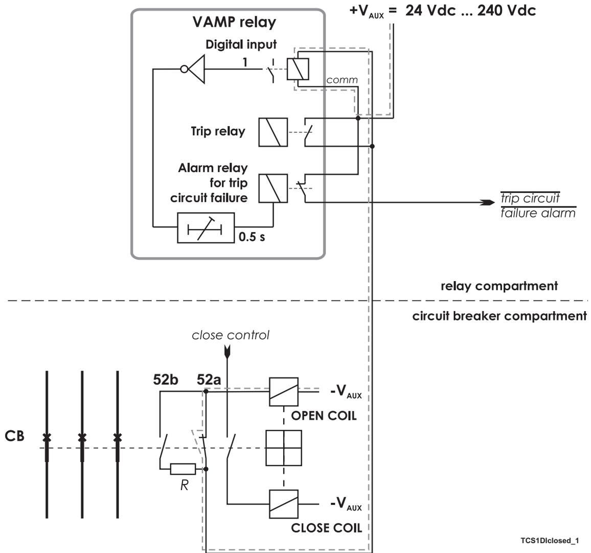
Figure 10.2: Trip circuit supervision using a single digital input and an external resistor R. The circuit-breaker is in the closed position. The supervised circuitry in this CB position is double-lined. The digital input is in active state when the trip circuit is complete.
