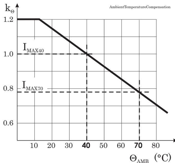
Figure 5.19: Ambient temperature correction of the overload stage T>.
