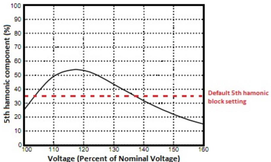
Figure 5.40: Harmonic content of transformer exciting current as a function of the applied voltage
