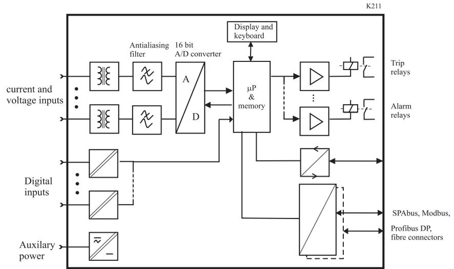
Figure 4.1: Principle block diagram of the VAMP hardware
