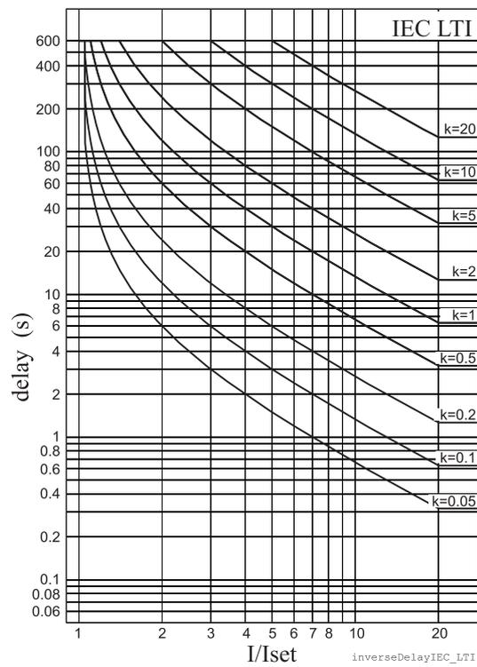
Figure 5.46: IEC long time inverse delay.
