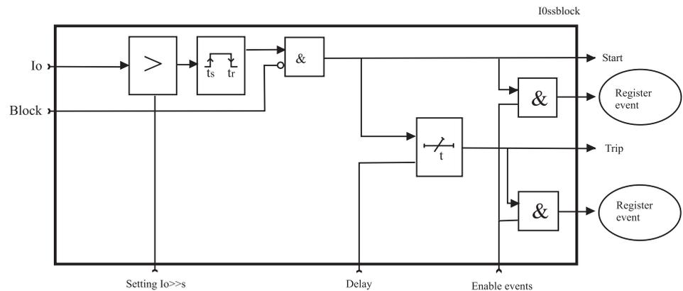
Figure 5.14: Block diagram of the earth fault stages  $I_0 >>$ ,  $I_0 >>>$ ,  $I_0 >>>>$
