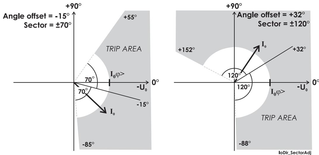
Figure 5.12: Two example of operation characteristics of the directional earth fault stages in sector mode. The drawn  $I_0$  phasor in both figures is inside the trip area. The angle offset and half sector size are user's parameters.
