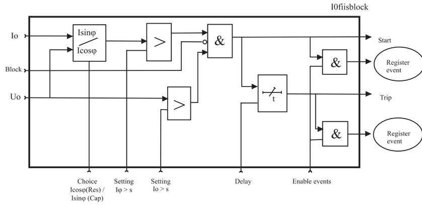
Figure 5.10: Block diagram of the directional earth fault stages  $I_{0\phi} >$ ,  $I_{0\phi} >>$
