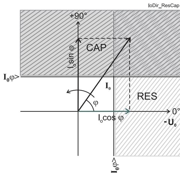
Figure 5.11: Operation characteristic of the directional earth fault protection in Res or Cap mode. Res mode can be used with compensated networks and Cap mode is used with ungrounded networks.
