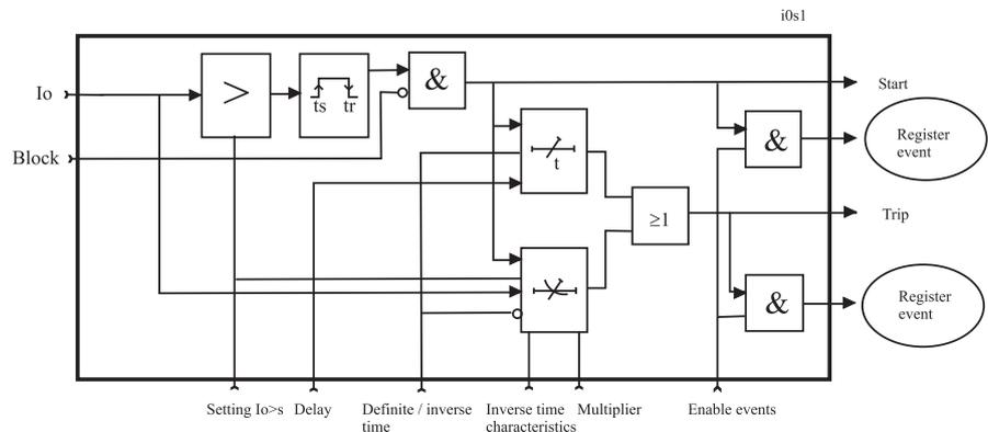
Figure 5.13: Block diagram of the earth fault stage  $I_0 >$
