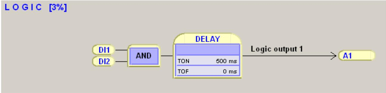
Figure 10.11: An example of logic configuration for trip circuit supervision with two dry digital inputs DI1 and DI2.
