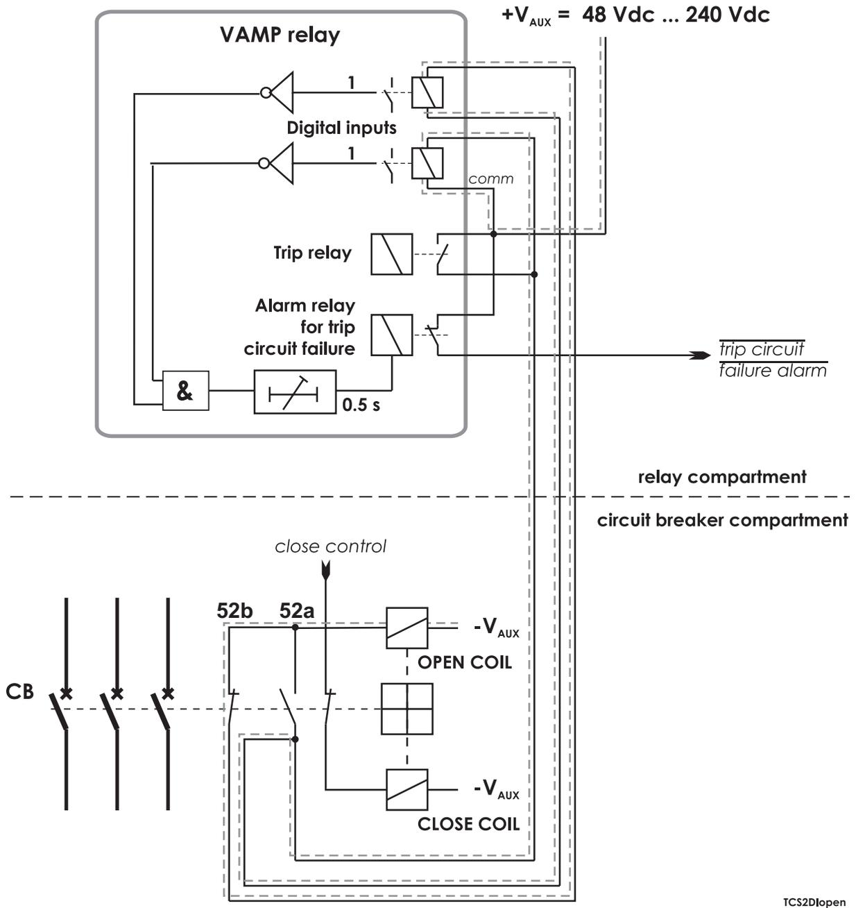
Figure 10.9: Trip circuit supervision with two digital inputs. The CB is in the open position. The two digital inputs are now in series.
