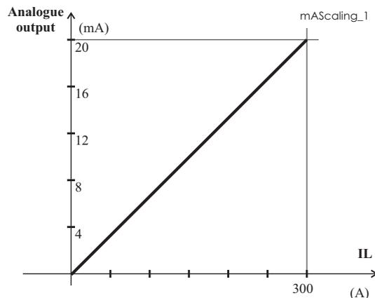
Figure 7.3: The average of the three phase currents. At 0 A the transducer output is 0 mA, at 300 A the output is 20 mA
