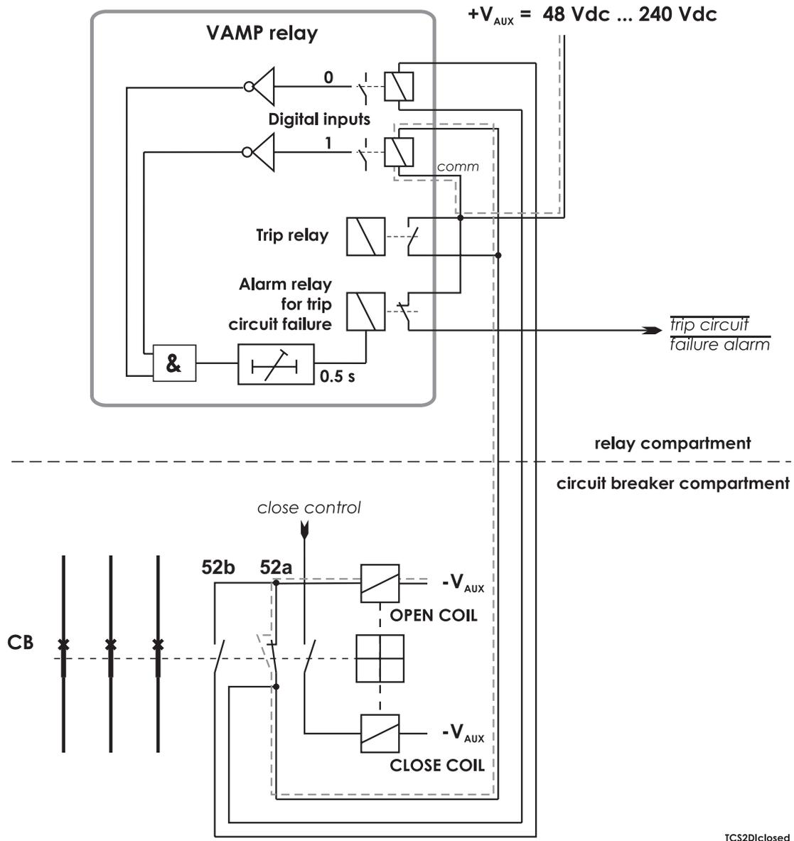
Figure 10.8: Trip circuit supervision with two digital inputs. The CB is closed. The supervised circuitry in this CB position is double-lined. The digital input is in active state when the trip circuit is complete.
