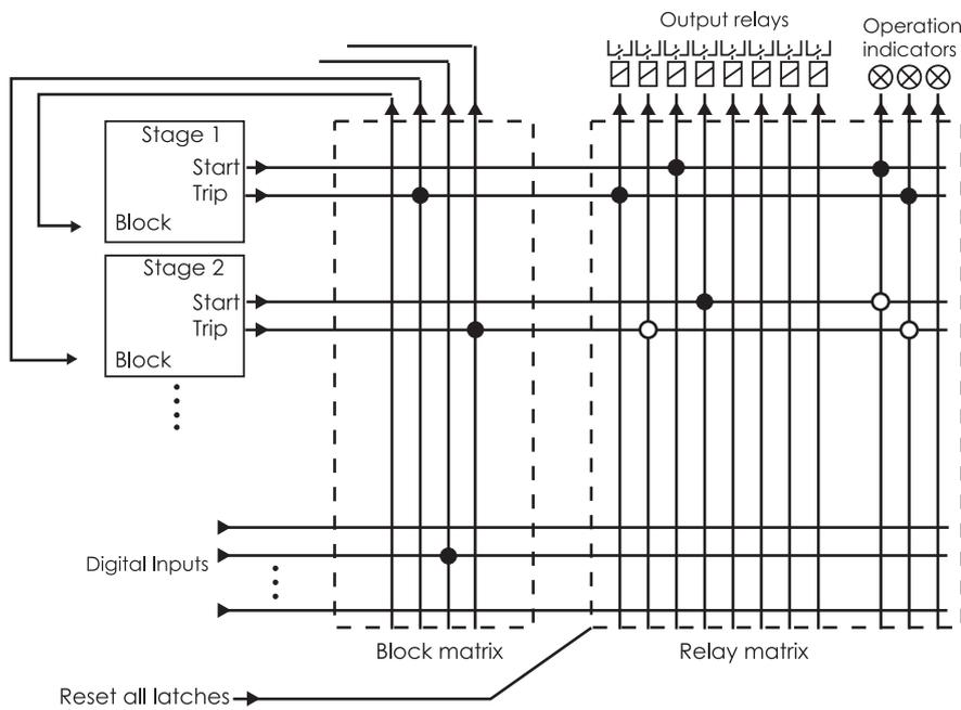
Figure 8.5: Blocking matrix and output matrix
