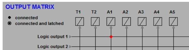
Figure 10.12: An example of output matrix configuration for trip circuit supervision with two digital inputs.
