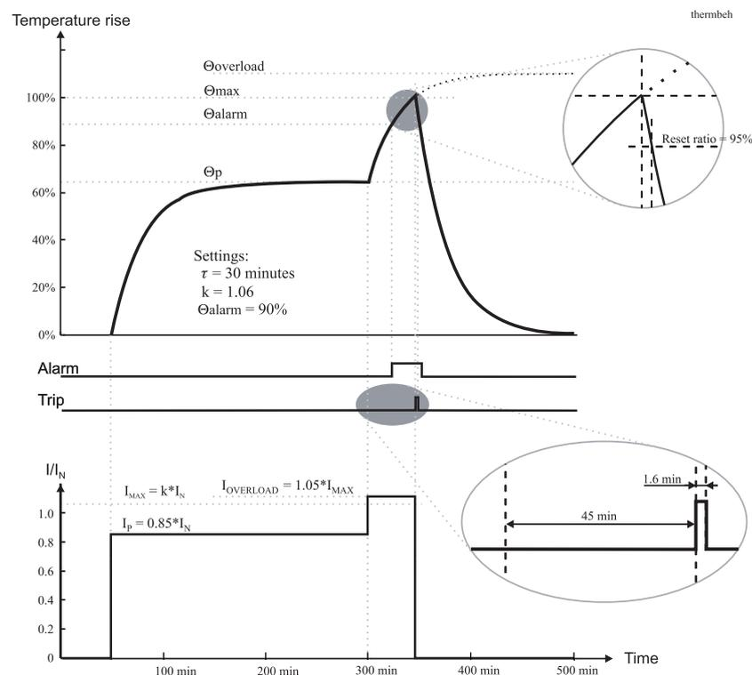
Figure 5.20: Example of the thermal model behaviour.
