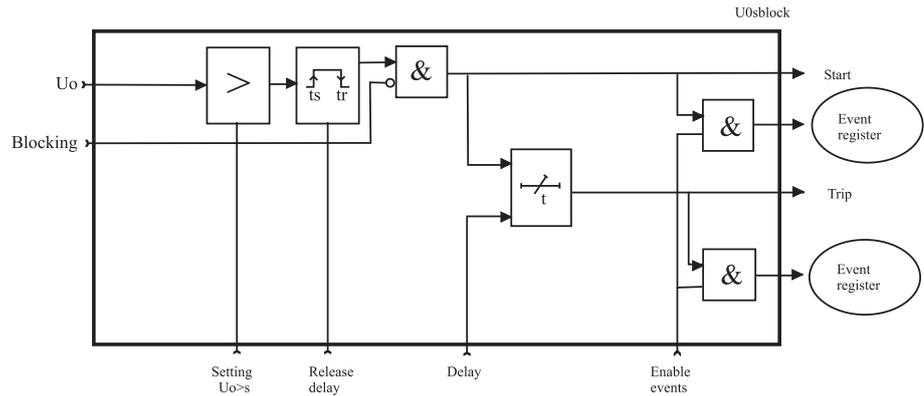
Figure 5.18: Block diagram of the zero sequence voltage stages  $U_0>$ ,  $U_0>>$
