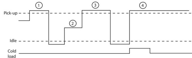
1. No activation because the current has not been under the set  $I_{DLE}$  current.
