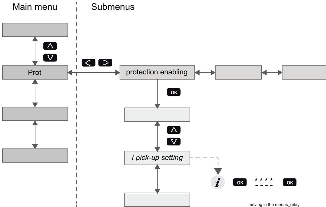
Figure 2.3: Moving in the menus using local HMI
