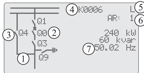
Figure 2.1: Sections of the LCD dot matrix display
