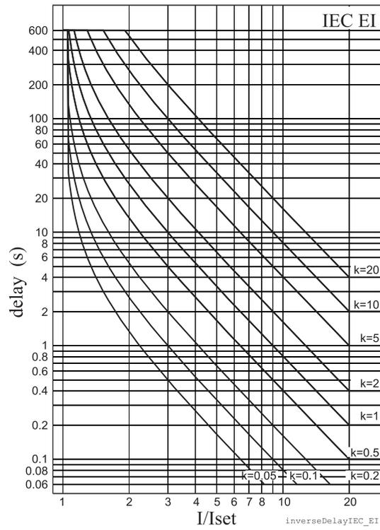
Figure 5.44: IEC extremely inverse delay.
