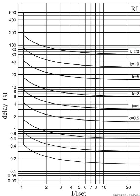
Figure 5.57: Inverse delay of type RI.
