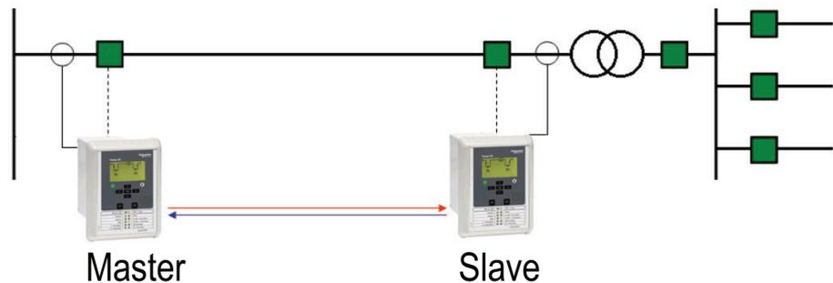
Figure 10.1: Line differential protection and auto-reclosing
