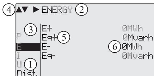
Figure 2.2: Sections of the LCD dot matrix display
