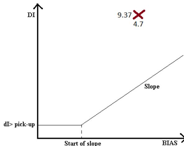
Figure 5.24: Example BIAS and differential calculation
