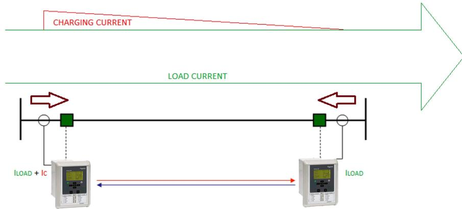
Figure 5.35: Behaviour of constant charging current
