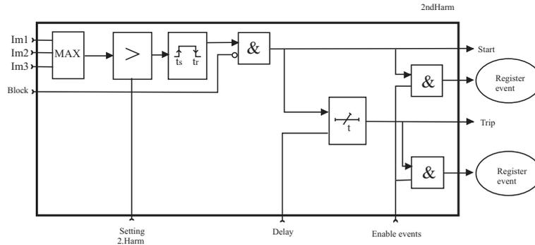
Figure 5.21: Block diagram of the magnetising inrush stage.
