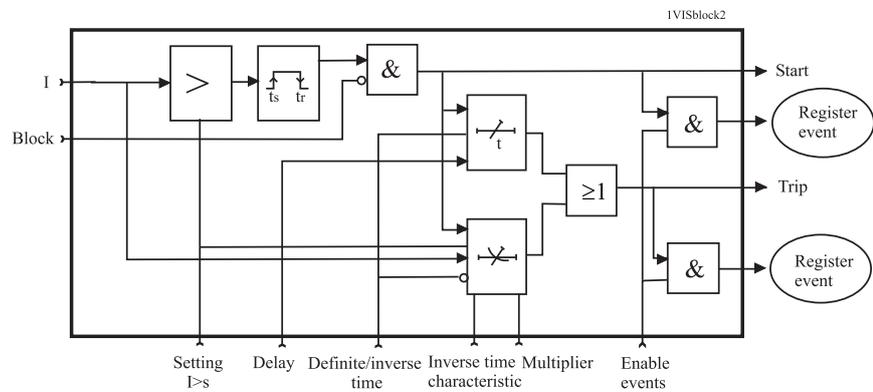
Figure 4.3: Block diagram of a basic protection function
